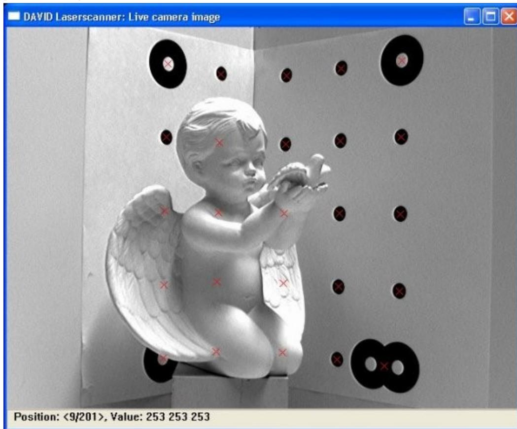
2. Switch on the laser and point it into the scene. Use the button for camera settings above the Pause button to adjust the camera settings (aperture, exposure), the position of the laser, and the light conditions in your room so that the laser line is clearly and brightly visible in the image, while the rest of the image is as dark as possible:
