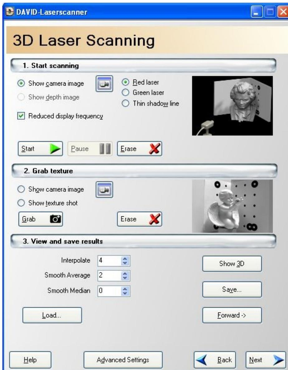
After calibrating the camera (see [Camera Calibration](#)) you can start scanning. The following steps will guide you through the 3D laser scanning dialog of DAVID:
